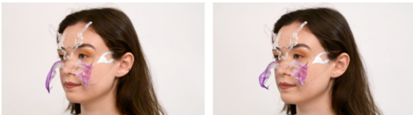
Figure 1: A model wearing the Social Prosthesis headpiece, nosepiece, and touch-sensing temporary tattoo. When the temporary tattoo is triggered through touch contact, the nose-piece starts curling in reaction.
